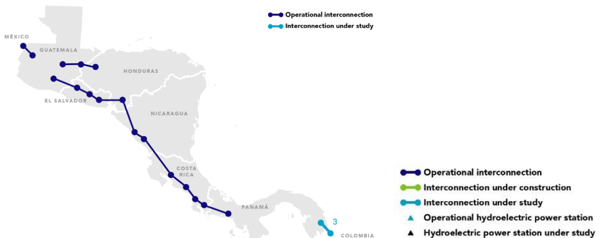
Figure 2. Regional electricity links in Central America
