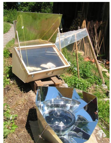
A Sun Oven box cooker uses reflective panels to concentrate sunlight, cooking food without emissions. Accessed 12 June 2014: http://upload.wikimedia.org/wikipedia/commons/e/e0/FOUR_SOLAIR_E_SUN_OVEN_HORNO_SOLAR.JPG .
